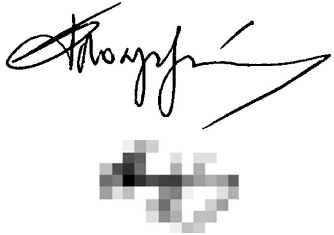
Fig. 4. The grid feature vector of a signature.
